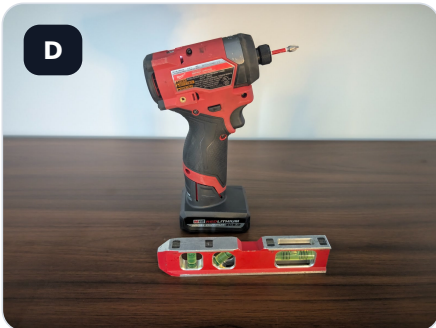
Drill, anchor sized bit, Phillips bit, and level.
